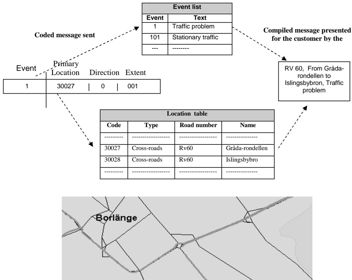
Figure. 5. The structure of a sent coded RDS-TMC message and how it is compiled
