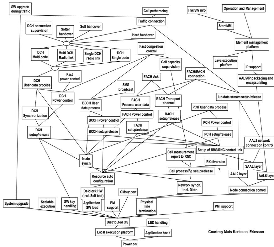
Fig. 6 The anatomy of the central processor
