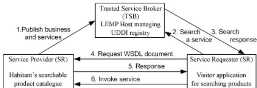
Fig. 3, An illustration of Web Service use in a LEMP setting.
