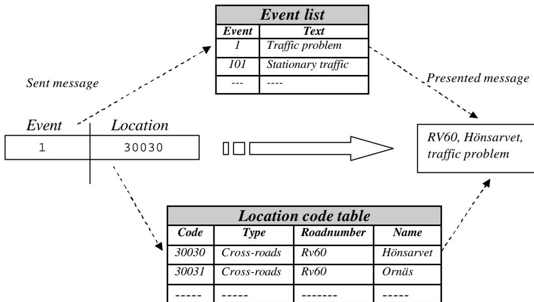
Figure 8. The transfer of an RDS-TMC traffic message
