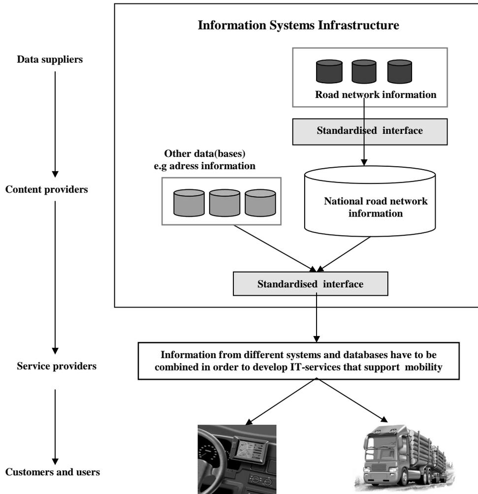
**Figure 3.** The NVDB is a part of an ISI that is a prerequisite for a number of ITS-services
