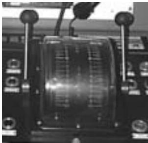
Fig. 2.9. The machine telegraph represents the desired state of the Object, the speed of the ship.
